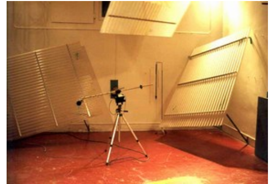
Figure 12. Barrier absorption: Reverberation Room Method photo #2553
